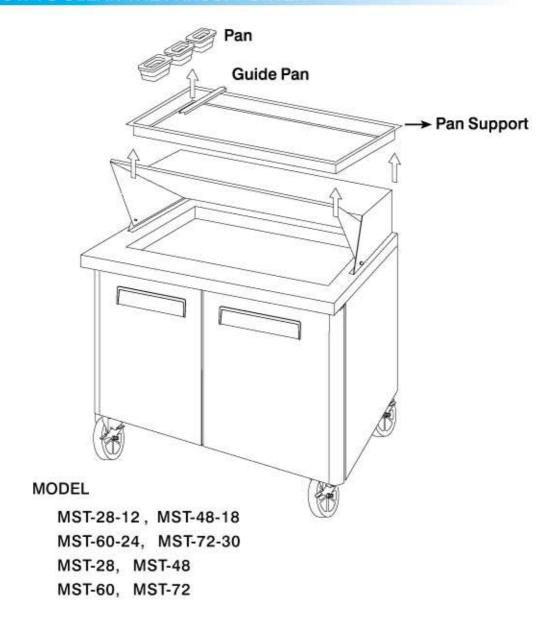
Remove the Guide Pans and Pans. Then pull out the Pan Supporter. Clean the pan supporter and reinstall in place.
