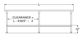
All units ship unassembled for reduced shipping cost. Units 7 ft. and larger are furnished with six legs. All dimensions are typical. Tolerance +/- .500".
